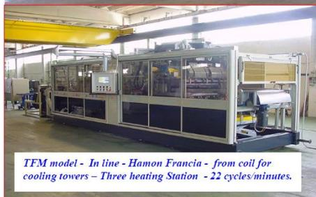
TFM model - In line - Hamon Francia - from coil for cooling towers – Three heating Station – 22 cycles/minutes.
