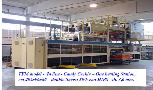
TFM model - In line - Candy Cechia – One heating Station, cm 206x96x60 – double liners: 80/h con HIPS - th. 3,6 mm.
