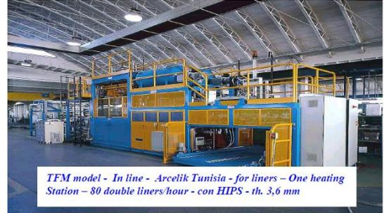
TFM model - In line - Arcelik Tunisia - for liners – One heating Station – 80 double liners/hour - con HIPS - th. 3,6 mm
