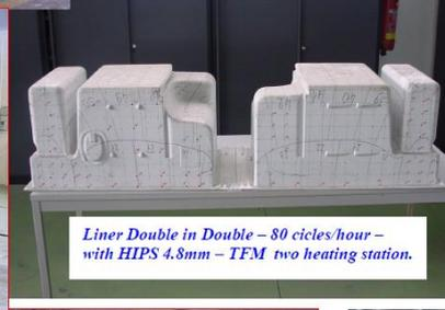
Liner Double in Double – 80 cycles/hour – with HIPS 4.8mm – TFM two heating station.
